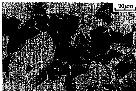
Fig. 6 Surface topography of annealed specimen after fatigue ( \sigma=300 MPa, N=3 \times 10^5 )
