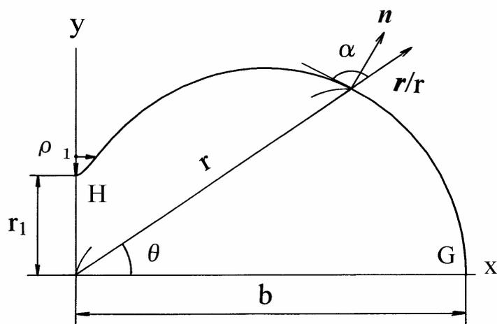
Fig.2 Geometry of the sintering particle. The arrows near the grain boundary indicates the diffusion paths of atoms.  $r/r$  is the unit vector,  $n$  is the unit vector normal to the shape profile, and  $\tan \alpha = r/r$  where  $r = dr/d$ .
