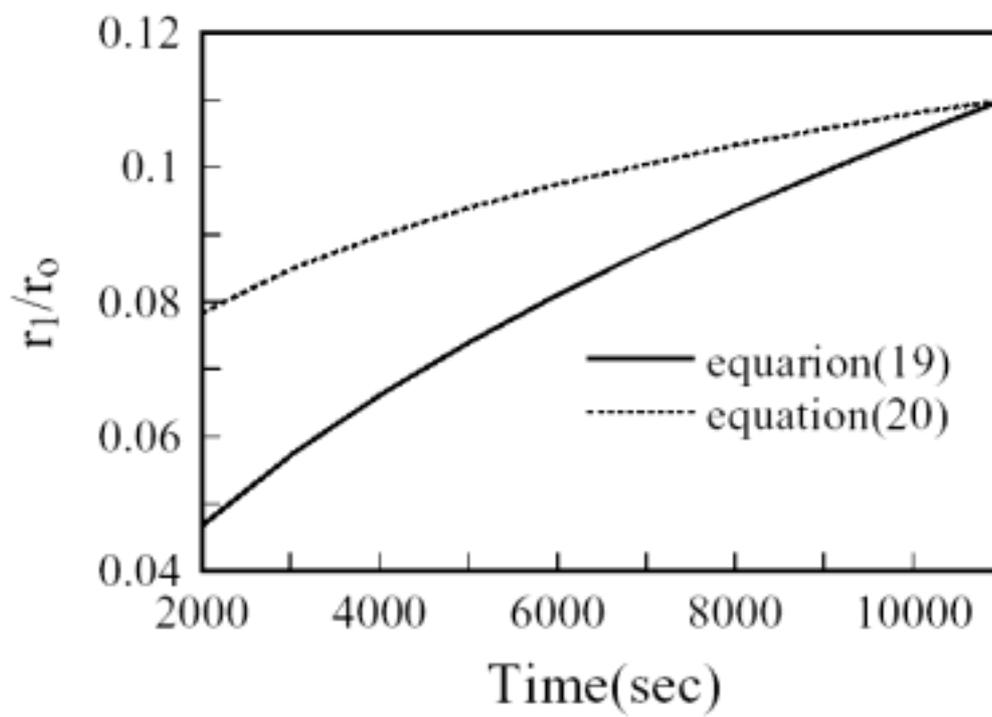
Fig.3 Numerical comparison of two kinds of the neck growth equations for copper wires by lattice diffusion.
