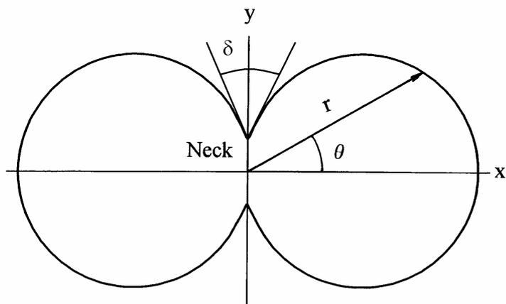
Fig. 1 Illustration of the geometry of the two cylindrical particles in two dimension.
