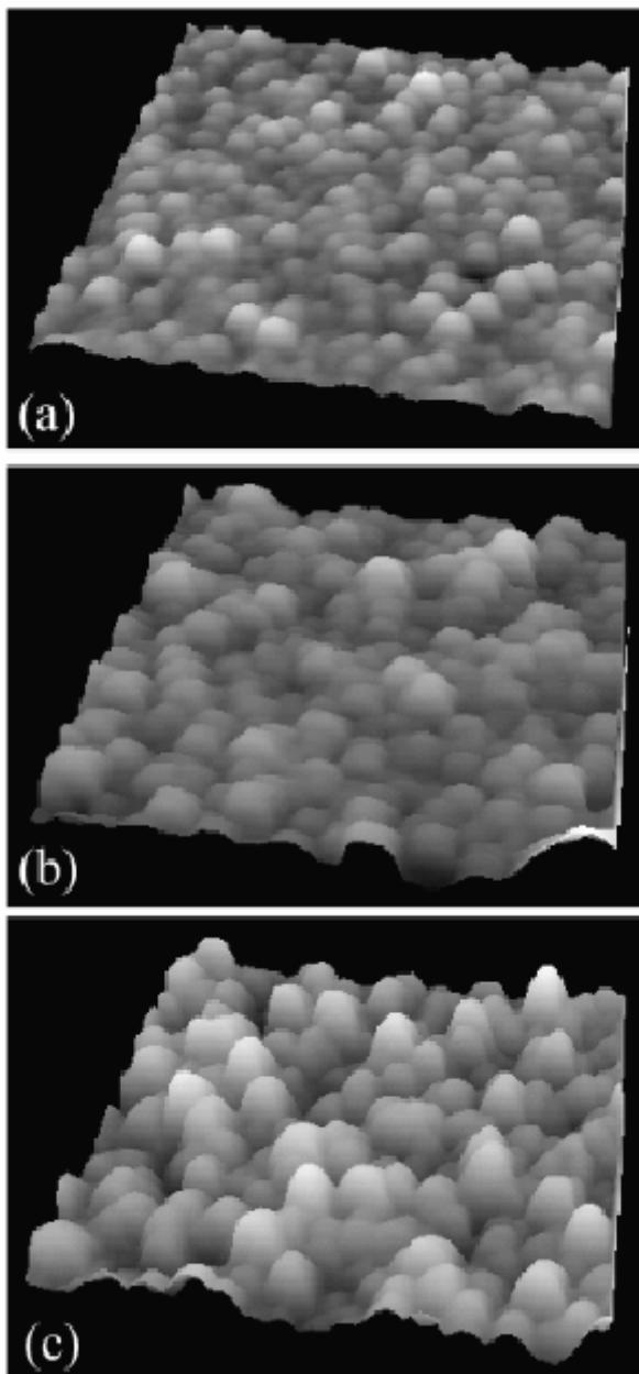
**Fig.1** AFM images of the nickel films grown at a low current density of  $2\text{mA/cm}^2$  for (a) 200, (b) 500 and (c) 800sec. Each image size is  $2000\times 2000\text{nm}^2$  and the vertical scale of each image with a resolution of  $512\times 512$  pixels was magnified by a factor of 3.6 in order to enhance viewing.
