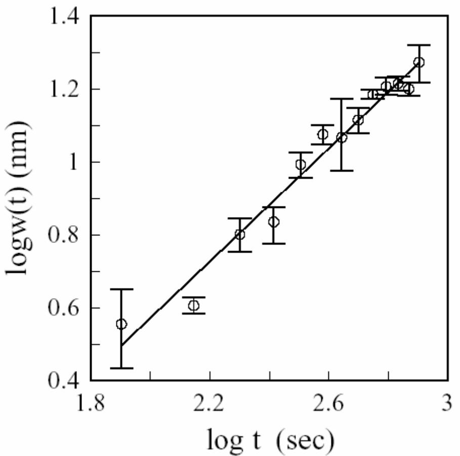
Fig.3 The scaling of the rms roughness  $w(t)$  with time, calculated from the AFM images of the electrodeposited nickel films at 323K. The slope of the best fitting line is  $\beta=0.78 \pm 0.03$ .
