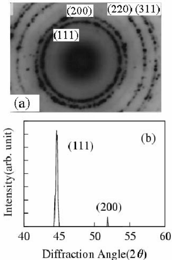
**Fig.4** Electron and X-ray diffraction patterns of the electrodeposited nickel films. (a) the incident electron beam operated at an accelerating voltage of 160kV was perpendicular to the surface of the nickel film grown for 440sec. (b) the X-ray CuK $\alpha$  was scattered by the nickel films grown for 1500 sec using a standard 0-2θ diffractometer.
