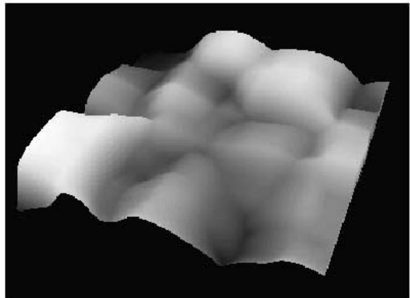
Fig.5 The AFM image of the nickel mounds on the ITO glass that have preferred crystallographic planes. The image size is 500x500nm<sup>2</sup>.
