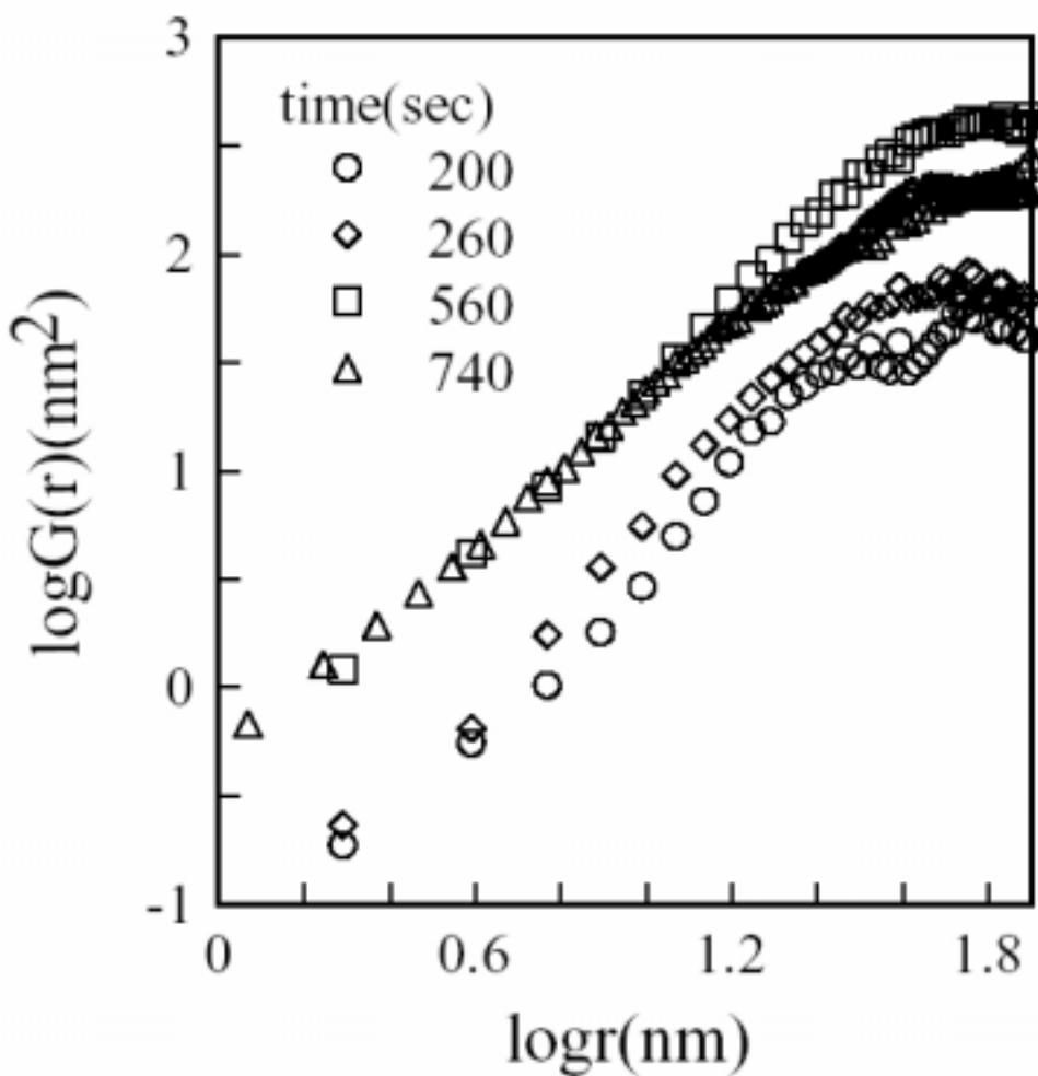
Fig.2 Log-log plot of the height-difference correlation functions  $G(r,t)$  vs  $r$ , calculated from the AFM images of the electrodeposited nickel films.
