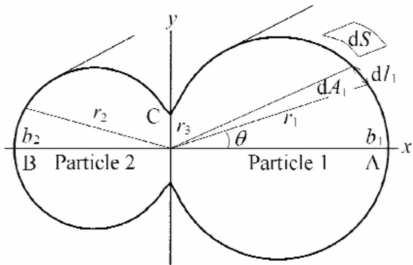
Fig. 1 Illustration of the geometry of the two cylindrical particles.
