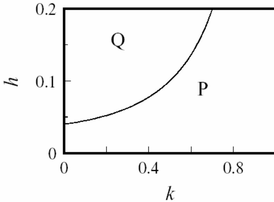
**Fig.2** Diagram of the size difference effect on the neck growth rate. The line indicates  $h(1-k)/(1+k^2)=0.04$ . P : area that has no effect on the growth rate, Q: area that has effect on the growth rate.
