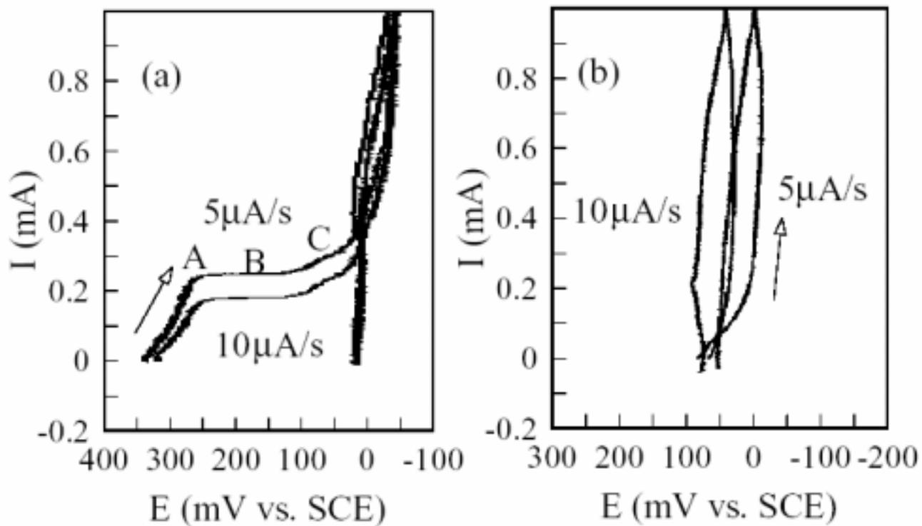
Fig.2 Cyclic current-potential curves at various scan rates of current for the two different concentration of lead acetate trihydrate in the electrolytes. (a) in the case of the electrolyte A free of lead acetate trihydrate, (b) in the case of the electrolyte B containing lead acetate trihydrate 0.2m mol/L.
