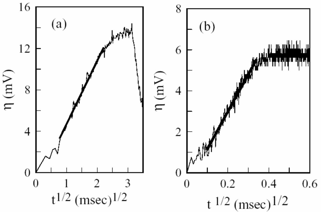
Fig.4 Plots of potential vs.  $t^{1/2}$  for the two different concentration of lead acetate trihydrate in the electrolytes. The straight lines best fitted to the experimental data are shown. (a) in the case of the electrolyte A: lead acetate trihydrate 0.0 mol/L, (b) in the case of the electrolyte B: lead acetate trihydrate 0.0002 mol/L.
