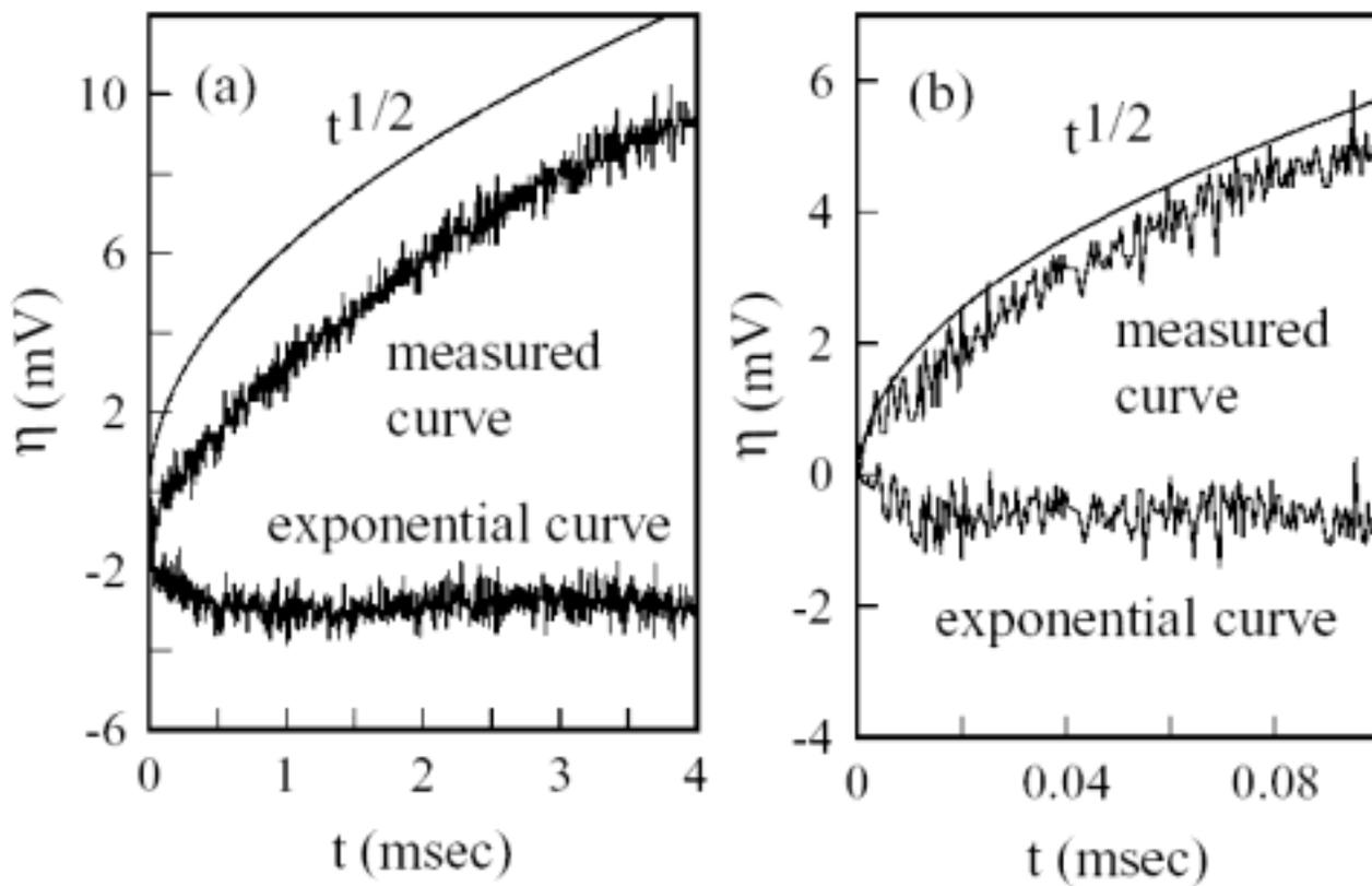
Fig.5 Plots of  $t^{1/2}$  and exponential curves determined from the measured potential-time curves in Fig.3.
