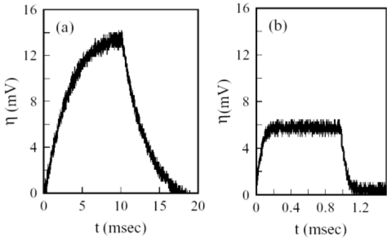
Fig.3 Typical potential-time curves for the multi-pulse currents. (a)  $i_t=0.0625\text{mA/cm}^2$  and  $T_h=10\text{msec}$  for the electrolyte A free of lead acetate trihydrate, (b)  $i_t=1.79\text{mA/cm}^2$  and  $T_h=1\text{msec}$  for the electrolyte B containing lead acetate trihydrate.
