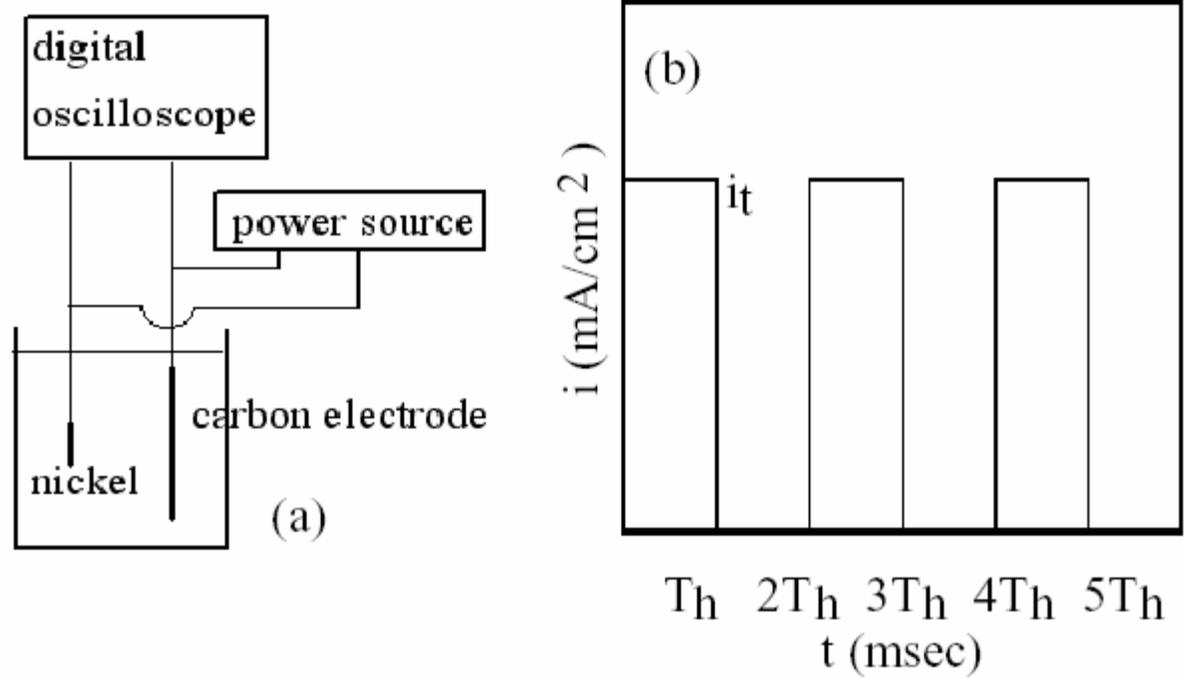
Fig.1 Schematic diagram for measurements of transient potential curves for multi-pulse currents applied across the electrodes. The current densities were chosen to hold the rising potential between the nickel and carbon electrodes at millivolts.
