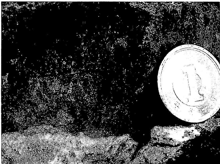
Fig. 3. Photographs of fault slickenside. (a) Slickenside observed within the Ryukyu Group (limestone), in Miyako island. (b) Slickenside observed within the Nosoko Formation, in Ishigaki island.
