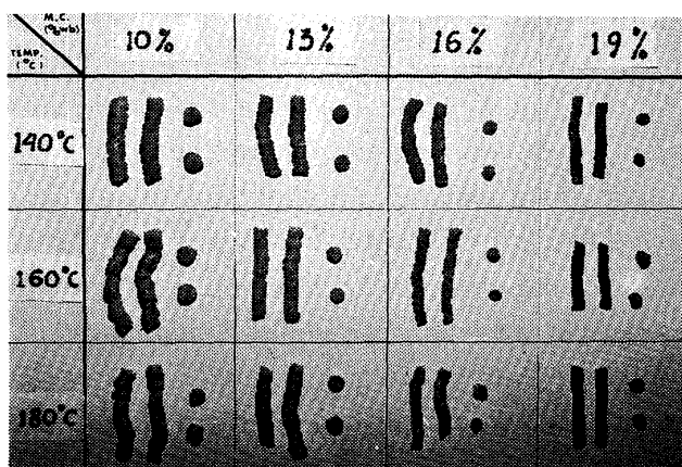
Fig. 1. The effect of process temperature and feed moisture content on physical appearances of product.
