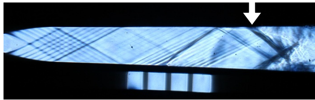
(b) Typical schlieren photograph for p_0/p_b=3.00
