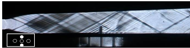
(b) Typical schlieren photograph for p_0/p_b=4.00
