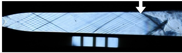
(b) Typical schlieren photograph for p_0/p_b=3.00
