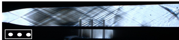
(b) Typical schlieren photograph for p_0/p_b=4.00
