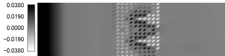
(d) Calculated velocity component normal to bottom wall
