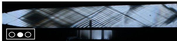
(b) Typical schlieren photograph for p_0/p_b=4.00
