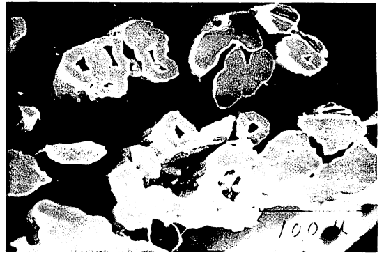
Fig. 4 Scanning electron micrograph of cross section of Ramie (Miyako jofu)
