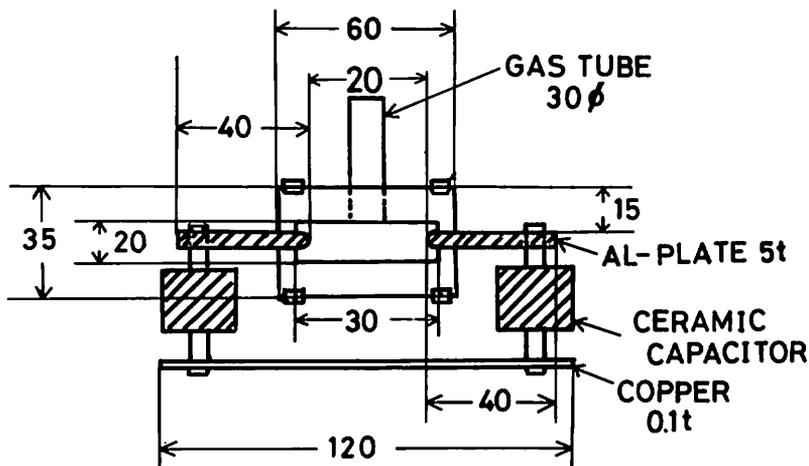
Fig.3 Cross section of the scaled-up  $N_2$  laser. The capacitors are arranged with separation of 4.3cm. The discharge electrodes are made of 5mm thick, 40mm wide and 930mm long aluminum plates.
