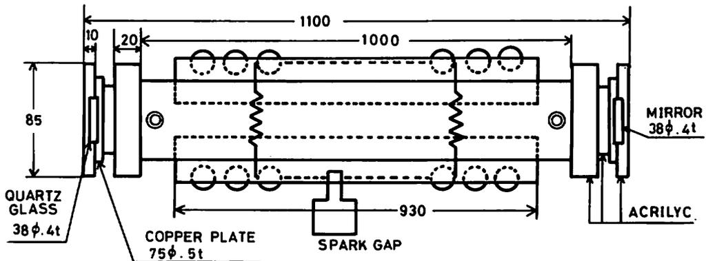
Fig.2 Top view of the scaled-up ceramic capacitor Blumlein-type  $N_2$  laser. It has an active length of 93cm, cross section of  $(3 \times 2)\text{cm}^2$ , electrode separation of 2.5cm and 44 (1000pF) capacitors.
