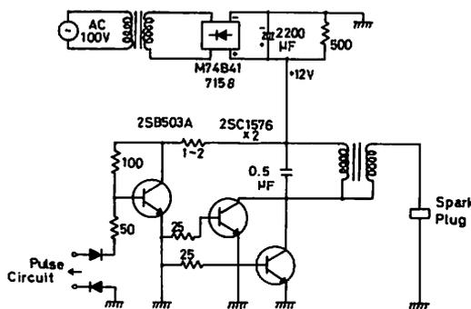
Fig.6 Ignition Coil Circuit.
