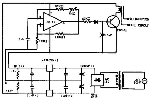
Fig.7 Pulse Circuit. The pulse rate is varied to a maximum pulse rate of 20Hz. The pulse circuit and ignition coil circuit are connected by a relay and form the trigger pulse circuit.
