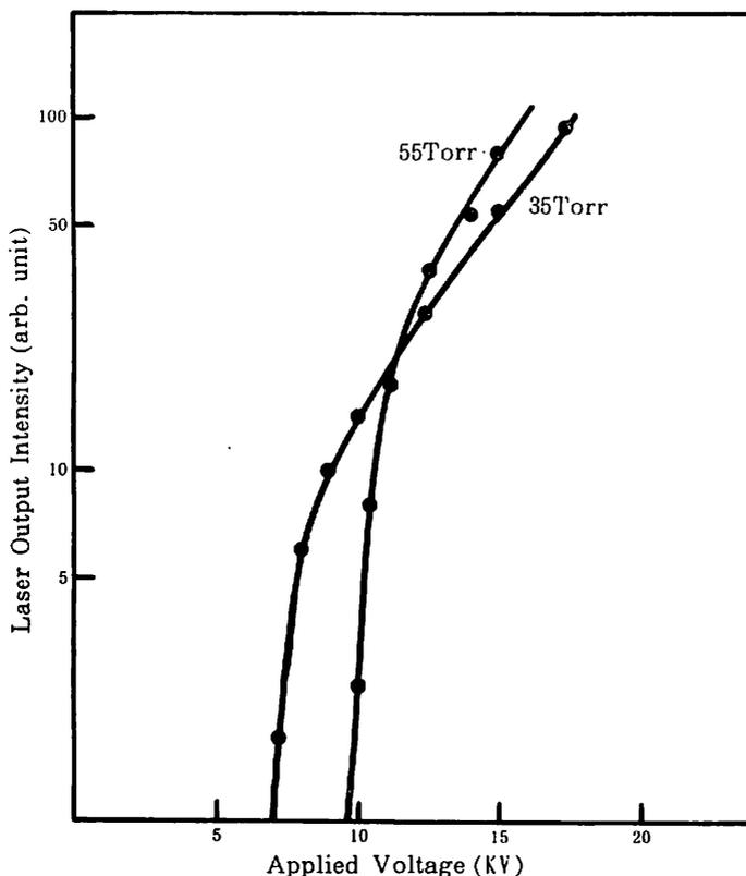
Fig.10 Laser output power versus charging voltage for pressure 55 and 35 Torr respectively. It is shown that the threshold increases as pressure increases and the output is proportional to the charging voltage.
