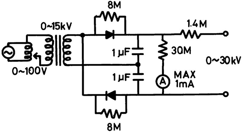
Fig.4 Power Supply Circuit. This gives a maximum output of 30KV using a 15KV neon transformer and voltage doubler. The output voltage is adjusted by a slidac.
