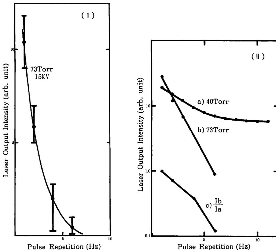
Fig.12 Output power as a function of pulse rate.
