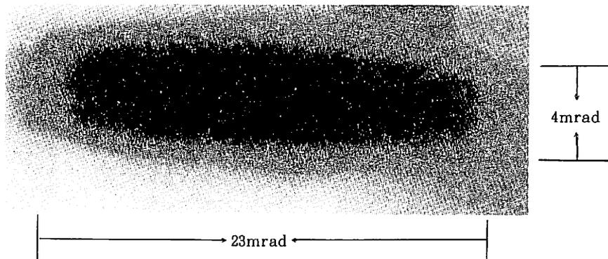
Fig.13 Far field pattern photograph of the laser output. The size is  $(9.2 \times 3.0)\text{cm}^2$  at a distance of 3m. The divergence is 4 mrad in the vertical and 23 mrad in the horizontal plane.
