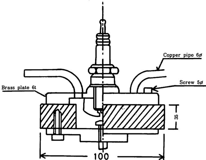
Fig.5 Detail of Spark Gap. The electrodes of the spark gap are made of brass and are rounded-off. The gap is adjusted by the lower screw.
