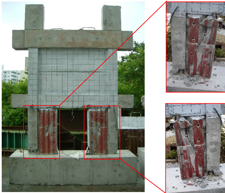
Fig. 2.15 Feature of the specimen R06P-WW after finishing loading test
