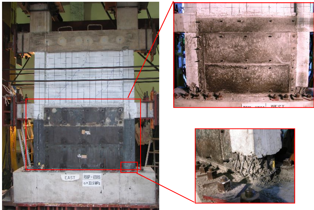
Fig. 2.21 Feature of the specimen R06P-PS after finishing loading test
