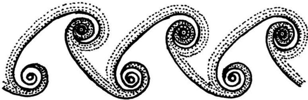
Fig. 2. Schematic diagram of fully developed vortices showing the transport of matter in a vortex street.
