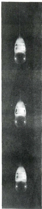
Fig. 5. Three successive pictures of a wake behind a sphere with three successive exposures.
