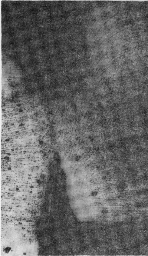
Photo 2 (a) Photomicrographs of the shear zone between Blank and scrap (a) in case of hollow groove
