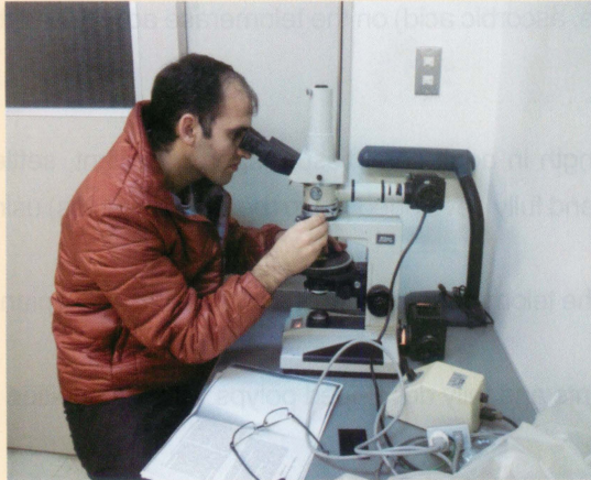
▲Observation of thin sections of rock samples by polarizing petrographic microscope.
