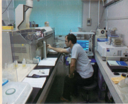
▲Analyses of bulk-rock chemical compositions for major and some trace elements by using the XRF spectrometer.
