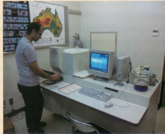
▲Measurement of trace and rare earth elements (REEs) by Inductively Coupled Plasma-Mass Spectrometer (ICP-MS).
