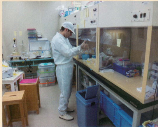
▲Preparing solution of acid-digested rock samples in the clean room for analyses of trace element and rare earth elements (REEs).
