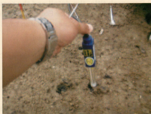
▲Figure3.Measuring TOC and TN on sediment
