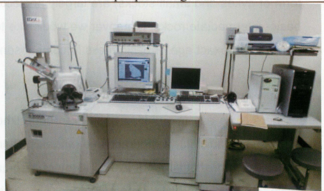
BSE images were obtained using a HITACHI S-3000N SEMicroscope.
