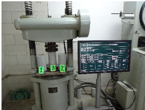
Fig. 6. Concrete samples for compressive testing.
