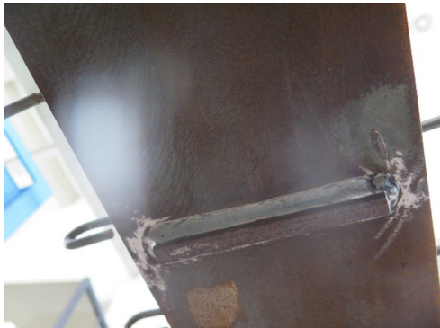
(c) Shear rib welded to the lower flange of the specimen.
