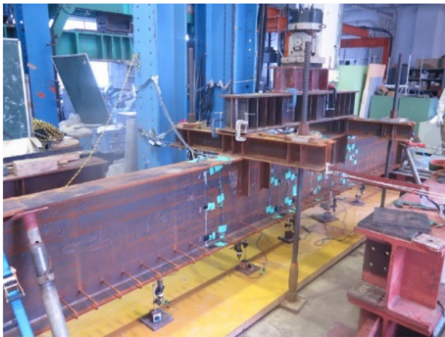
(b) Preflexion setup in laboratory.
