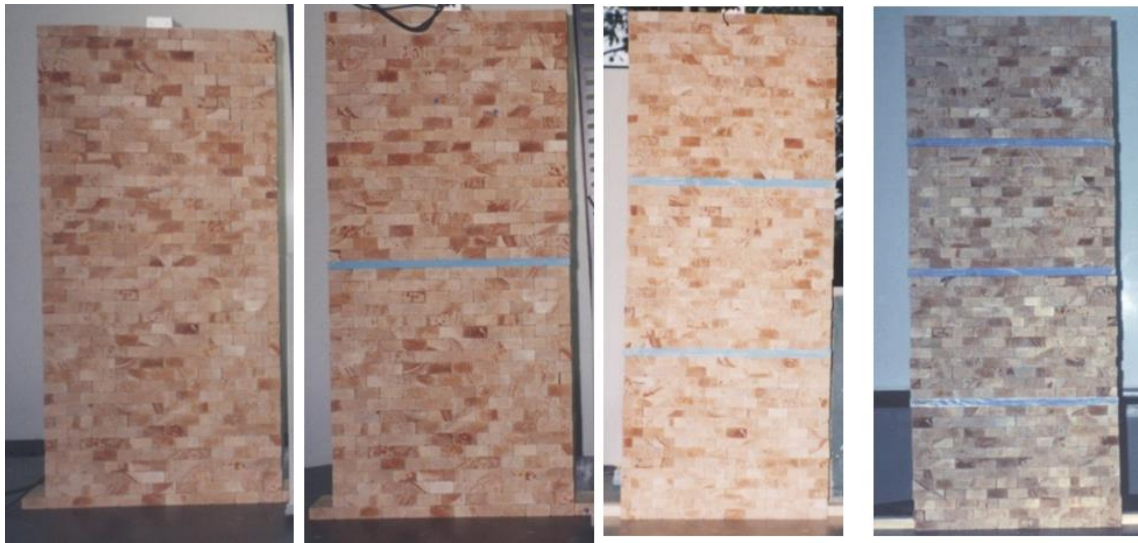
Figure 7.37 Views of the wooden masonry walls with different number of lintels.
