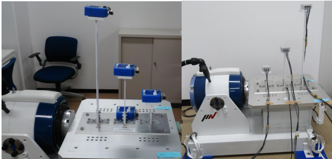
(a) Towers with wire-less accelerometers
