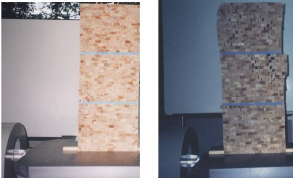
Figure 7.41 Views of the wooden masonry wall before and after shaking
