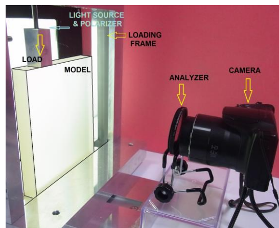
Figure 7.2 Implementation of photo-elasticity principle in practice, from (Aydan, 2020)
