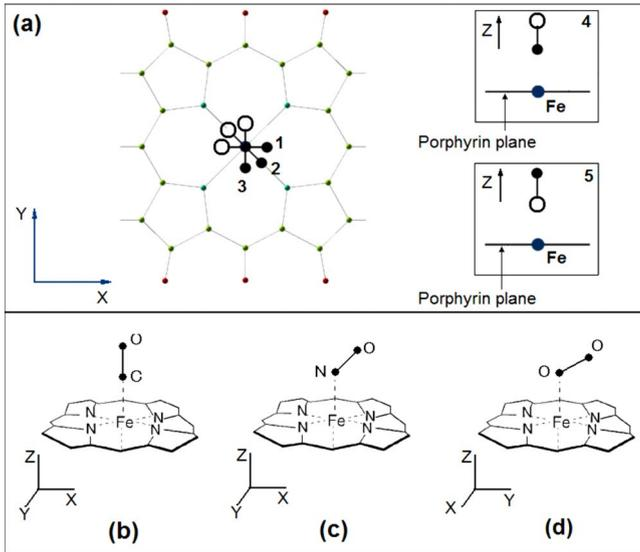
FIG. 3. (Color online) (a) Top view and side view of five initial adsorption sites of XO on FeTP and the structure for (b) CO-, (c) NO-, and (d) O<sub>2</sub>-adsorbed Fe tape-porphyrin after relaxing.
