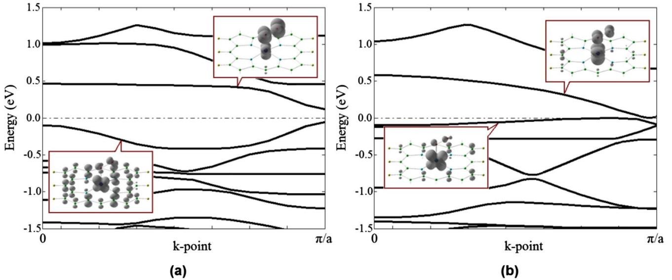
FIG. 9. (Color online) Band structures of (a) majority-spin and (b) minority-spin electrons for Fe tape-porphyrin with  $O_2$  adsorbed. Isosurface plots denote the electron charge density distribution of the conduction band and valence band near the Fermi level. The Fermi level was set to origin. The charge density is displayed at  $0.03 e/\text{\AA}^3$  isosurface value.
