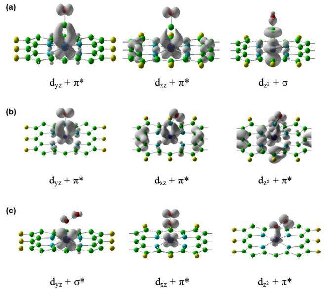
FIG. 5. (Color online) The partial (band decomposed) charge density at  $\Gamma$  point in the Brillouin zone of (a) FeTP-CO, (b) FeTP-NO, and (c) FeTP-O<sub>2</sub>, which describe the hybridization between  $d$  orbitals and  $\pi^*$  orbitals. The charge density is displayed at  $0.025 e/\text{\AA}^3$  isosurface value by VASP Data Viewer program.<sup>26</sup>
