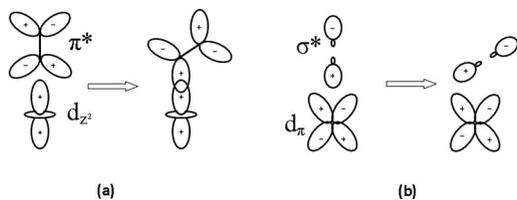
FIG. 4. The mechanism of forming the bent structure when the diatomic molecules bind to the iron tape-porphyrin. Here,  $d_{\pi}$  implies  $d_{xz}$  or  $d_{yz}$ . For the NO case, the first process ( $d_{z^2} + \pi^*$ ) is shown. However, in the case of O<sub>2</sub>, both processes are included. This is the main factor that leads to the differences in the Fe-X-O angle.
