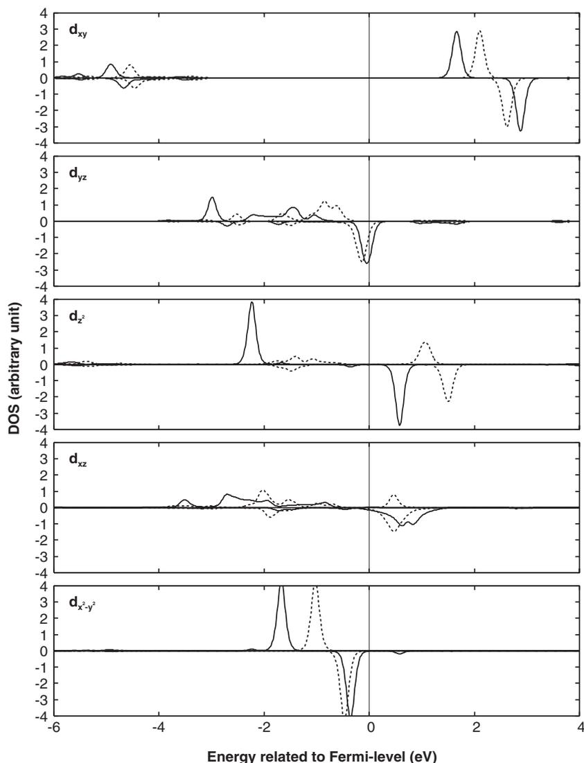
FIG. 8. The partial density of states of  $3d$  orbitals of the Fe atom in FeTP (solid line) and FeTP-O<sub>2</sub> (dash line). In all subfigures, the unit for DOS is arbitrary and the unit for energy is eV. For each subfigure, the upper and the bottom panels correspond to spin-up and spin-down electrons, respectively. The Fermi level is shifted to zero.
